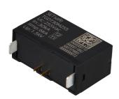
Thermally Protected Gas Discharge Tube (TGDT) is a gas discharge tube (GDT) combined with thermal protection. When GDT takes function and discharged for a certain number of times, the internal insulation performance decreases as well as the follow current interrupting ability, eventually leading to GDT short circuit failure. TGDT can make GDT disconnect from the circuit through thermal trip when the GDT degrades or short-circuit fails.
